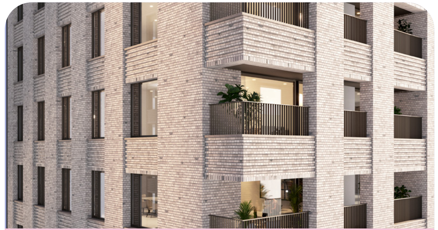
High quality brick construction with a mix of different brick laying patterns to add texture on all towers
